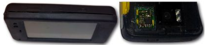
Figure 1: The outward appearance of ForcePhone covered with a silicone case and the embedded FSR.
